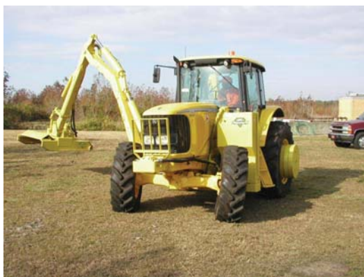
Dr. Joe Neal and Dr. Jim Burton of NC State University's Horticulture Science Department conducted research on using the Diamond Wet Blade (photo, left) and Brown Brush Monitor (photo, right) mower and herbicide applicator systems for more effectively controlling invasive woody plants along NCDOT right-of-ways.
