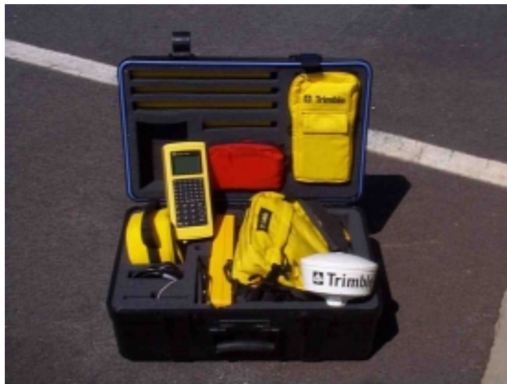
Figure 1. GPS Equipment- Data Logger, Antenna, and GPS Receiver in Backpack
