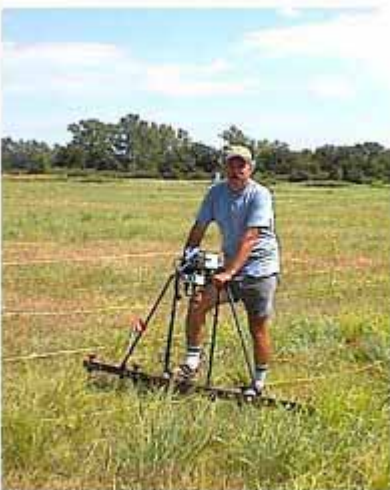
Geoscan Research RM-15/MPX-15 (electrical resistance)
